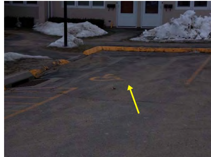
This designated parking space should be upgraded with a striped access aisle and a standing designation sign.
